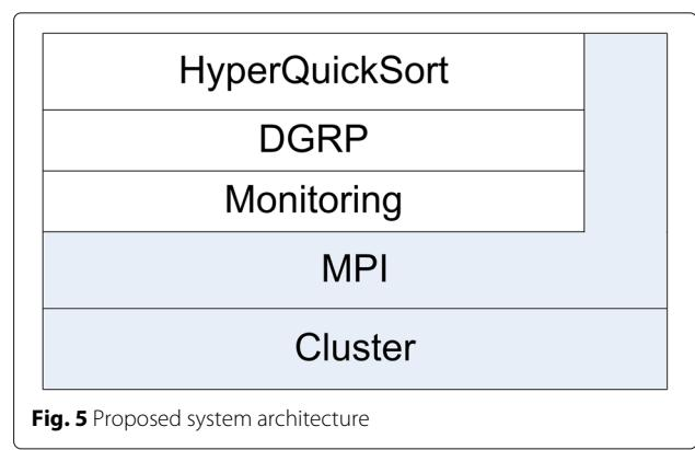
**Fig. 5** Proposed system architecture
