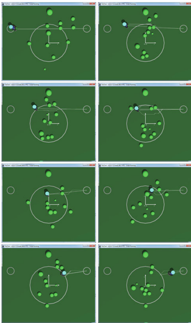
Fig. 20 Modified A* dynamic simulation results with discrete instants t = 1, 2, 3, 4, 5, 6, 7 and 8
