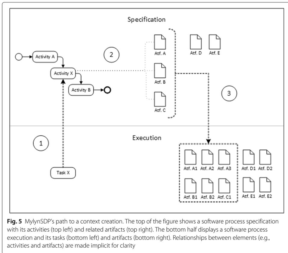
**Fig. 5** MylynSDP's path to a context creation. The top of the figure shows a software process specification with its activities (top left) and related artifacts (top right). The bottom half displays a software process execution and its tasks (bottom left) and artifacts (bottom right). Relationships between elements (e.g., activities and artifacts) are made implicit for clarity
