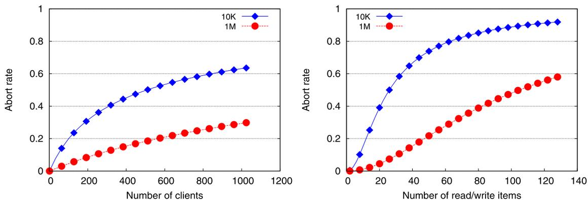
**Fig. 2** Abort rate versus number of clients (left) and number of items in a transaction (right) in the absence of byzantine clients
