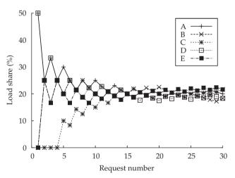
Figure 5. Cumulative load of slave nodes.
