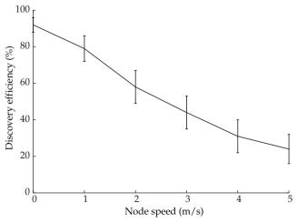
Figure 7. Discovery efficiency in a mobile scenario.
