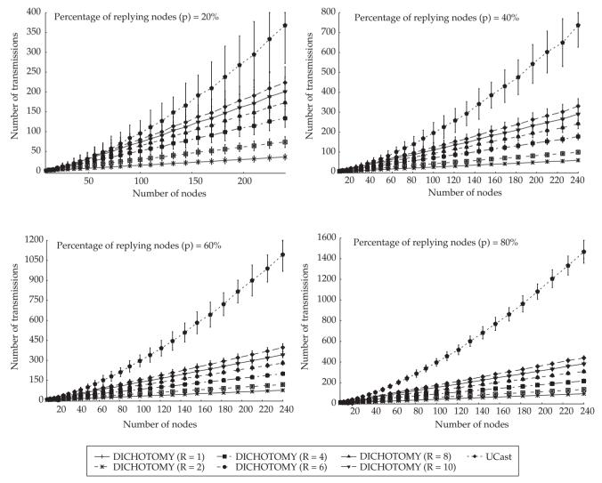
Figure 8. Network load in the mobile ad hoc grid due to reply messages.
