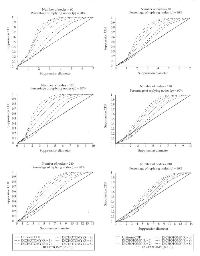
**Figure 9**. Distribution of reply suppressions (20% of replying nodes in the mobile ad hoc grid).
